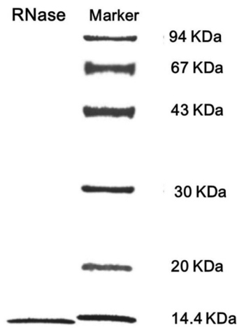
FIG. 3: SDS-PAGE results. Left lane: purified RNase. Right lane: molecular mass marker, from top downward: phosphorylase b (94 kDa), bovine serum albumin (67 kDa), ovalbumin (43 kDa), lactate dehydrogenase (30 kDa), soybean trypsin inhibitor (20 kDa), and alpha-lactalbumin (14.4 kDa).
